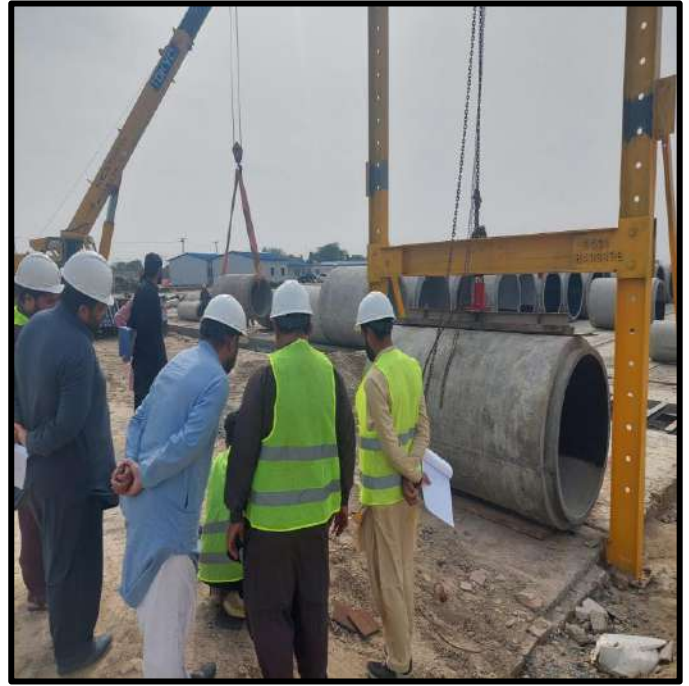
Picture 44: 03-Edge Bearing Test
