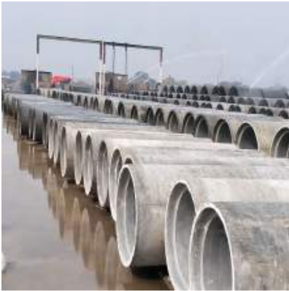
Picture 25: RCC Pipe Curing Yard
