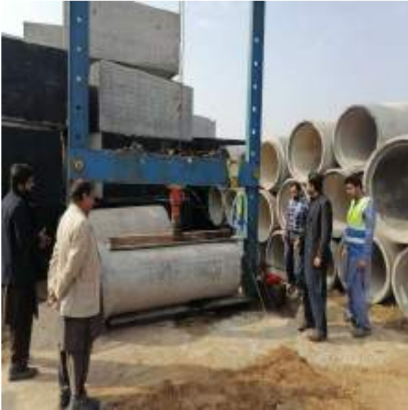
Picture 63: 3-Edge Bearing Testing for RCC Pipe
