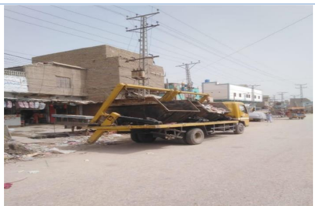
View of waste collection and transfer through Arm Roll Truck
