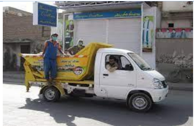
Minidumpers used for waste for waste collection in streets
